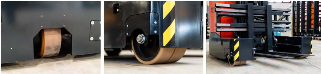
Different options for tyres make the truck extremely versatile: PU tyres are suitable for indoor use on industrial floors, PU SOFT tyres can be used both indoors and out, even on uneven floors and asphalt.
