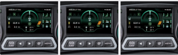
N (Normal) : Same acceleration feel as ICE forklifts H (High) : Implement instant acceleration performance for fast task processing E (Economic) : Smooth acceleration performance with energy efficiency
