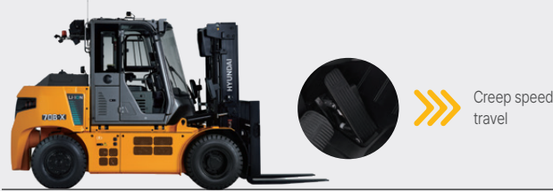
Allows travel at 2.5 km/h without pressing the accelerator
