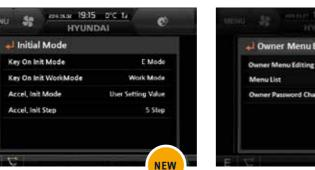
Key On Init Work Mode This feature allows operators to save the attachment mode setting so that the machine
