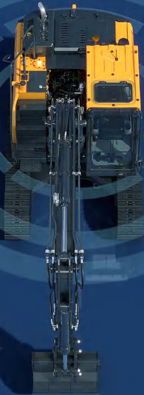
Secure field of vision in all directions through ten views including 3D bird's eye view and 2D/4CH view.
