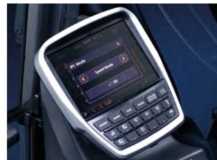
Intelligent Power Control
